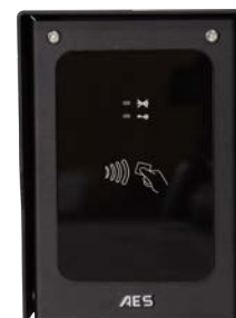
KEY-AUX-IBP-EU Aux unit with prox reader.
